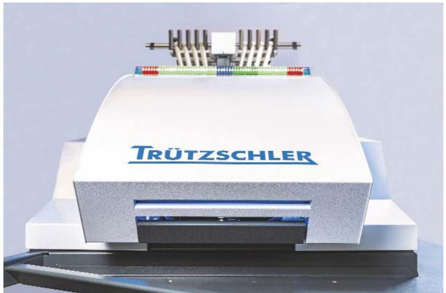
controlling an entire production process remotely - even with little staff. Intuitive human-machine interaction is provided by easy-to-remember lighting combinations. The employee knows instantly what the machine needs for further operation and can react accordingly. If, for example, he sees a yellow running light on the distant machine, he recognizes that new cans are needed. The operator immediately sets off with the empty cans.
