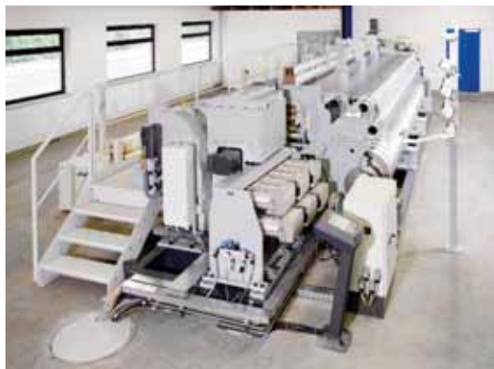
The Alpha Leantec machine from Stäubli, combined with the Unival 500 dobby for the production of 3D technical fabrics.
