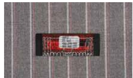
Front and rear views of a textile RFID label produced by Jakob Müller subsidiary TexTrace.
