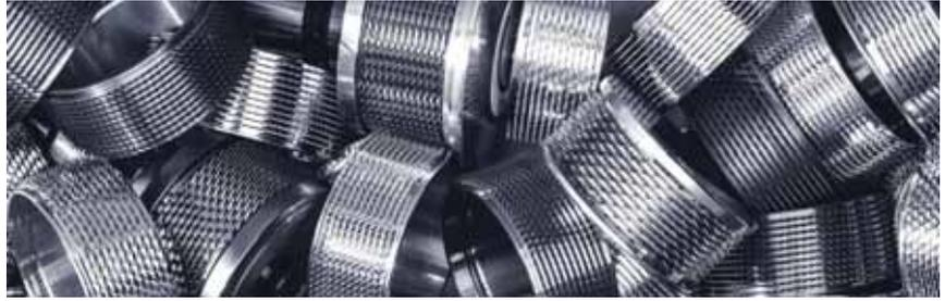
The product range of Trützschler Card Clothing also includes metallic wires for opening rolls.
