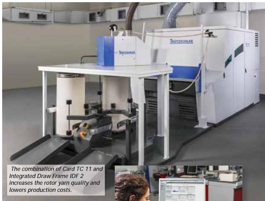
*The combination of Card TC 11 and Integrated Draw Frame IDF 2 increases the rotor yarn quality and lowers production costs.*
