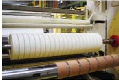
Inline slitting during winding is a speciality of Trützschler winders.
