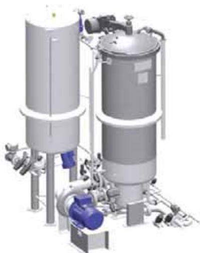
Depending on carry-over of the material, liquor ratios of 1:3.6 in partially flooded vessels are now possible in mill practice.
