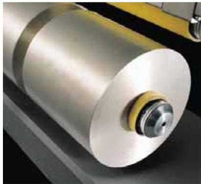
Precise package build up with winding heads for BCF and technical yarns.
