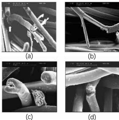
Figure 1: Dry abrasion morphology of untreated sample: (a) multiple split fibre end; (b) transversely and axially fractured; (c) rounded and axially split ends; (d) propagation of transverse fracture.
