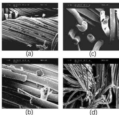
Figure 5. Dry abrasion morphology of Reaktant DH treated sample (a) surface damage and multiply splitted fibre ends, (b) stepped break, (c) rounded off and axially splitted fibre ends, (d) detail of fibres at the breaking point of yarn; mashed, mangled and twisted.
