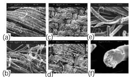
Figure 4. Fibrillation observed in untreated sample: (a) start of the fibrillation after first wash; (b) extensive fibrillation; (c) inner side of the crease; (d) outer side of the crease; (e) stepped break; (f) rounded fibre end.
