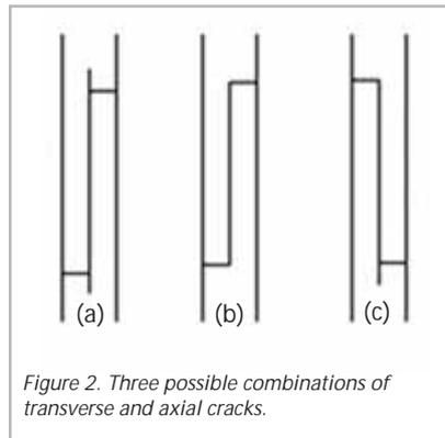
Figure 2. Three possible combinations of transverse and axial cracks.
