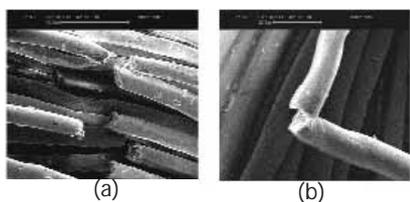
Figure 6. Fibre fracture observed in Reaktant FC treated samples: (a) brittle fractures at the crown; (b) brittle fracture through bending.
