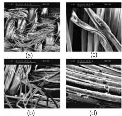
Figure 3. Morphology of fabric at the breakage point: (a) breakage of yarn; (b) detail of (a) mangled and axially split fibres; (c) detail of (a) crushed fibres; (d) smeared fibres at the yarn crown.
