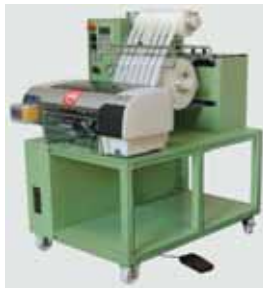
MDP2 MÜPRINT2 – the inkjet, direct printing system.
