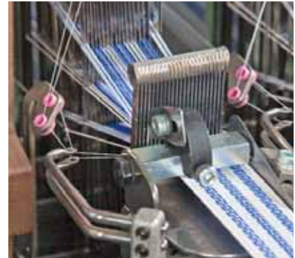
NH2 53 spaces with two-needle Z-system, weft insertion needles and auxiliary thread guide.
