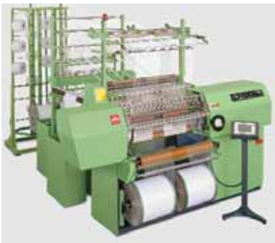
MDC 3/830E warp knitting machine (mechanically or electronically controlled) with weft insertion for elastic and non-elastic products.
