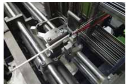
NH2M – narrow fabric needle loom for MultiSphere rope weaves.
