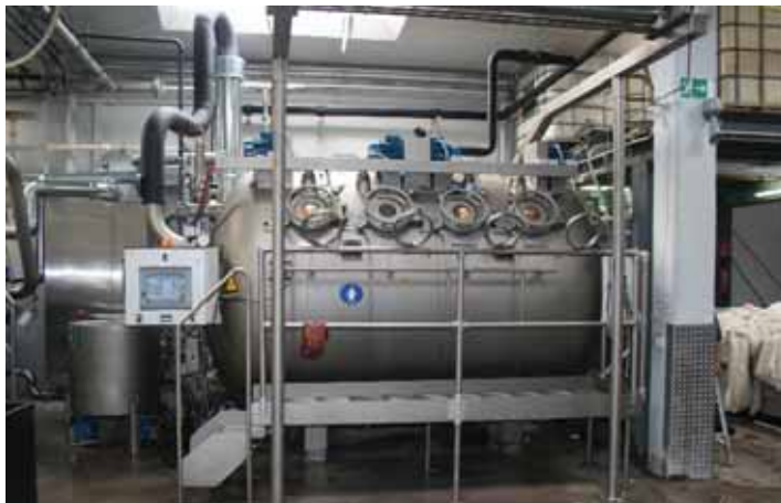
Thies 4-chamber iMaster H 2 O 140/4 dyeing unit.
