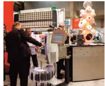
Gerard Küsters, head of Oerlikon Schlafhorst with the new Autocoro 8, which produced yarn at a rotor speed of 200,000 rpm.
