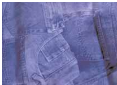
The transfer printing of natural fibres - the above picture shows two samples of 100% woven cotton garments with transfer printing effects,
