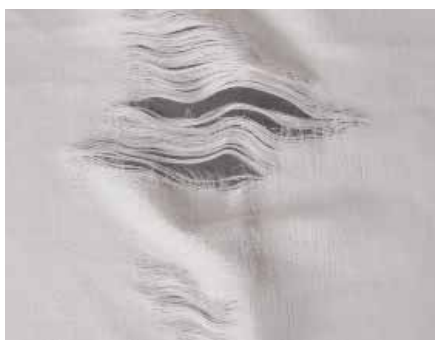
Result of insufficient abrasion resistance.
