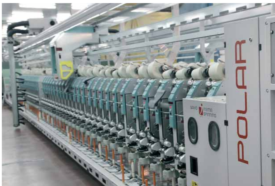
POLAR I/DLS- a new concept in automatic link winding.
