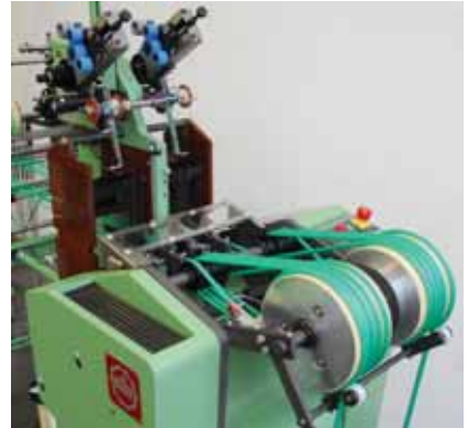
NG3M – narrow fabric needle loom for MultiSphere rope weaves.
