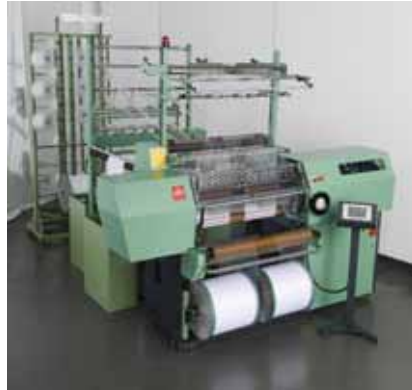
MDC 3/830 (with mechanical or electronic controls) – warp crochet knitting machine with weft insertion for elastic and non-elastic knits.
