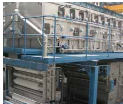
Knitcolora Pad Steam dyeing range by Goller.
