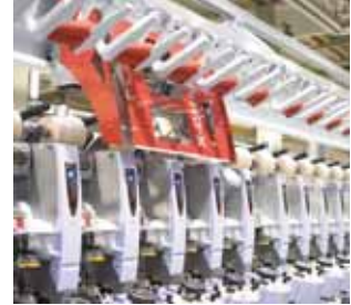
Fig 3: The new doffer X-Change for flexible automation.
