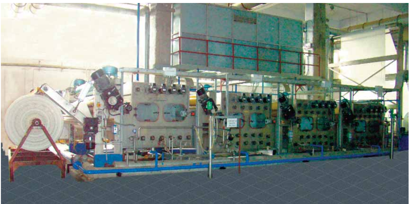
Open width washing machine by Menzel shown at the premises of Union Exports.
