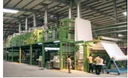
POWER-COLORTHERM / INFRATHERM Pad-Dry / Thermosol lines ensure an optimum dyeing and a crease-free fabric passage.
