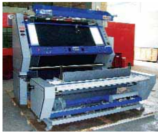
The fabric inspection machine Nazmatic for denim application.
