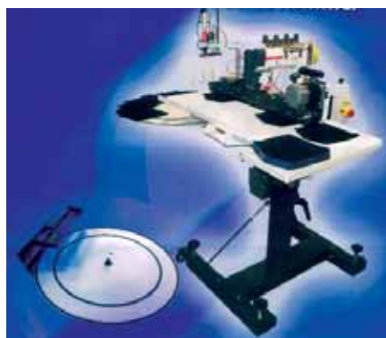
V700 - Automatic back pocket hemmer is one of the new unit Vibemac presented in 2009.
