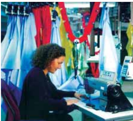
Eton Systems provide material handling systems consisting of overhead conveyor with individually addressable work stations.
