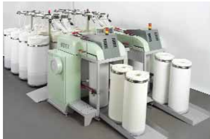
Fig. 1 New RSB-D 22 double-head autoleveler drawframe featuring a maximum delivery speed of 2 \times 1\,100 m/min.
