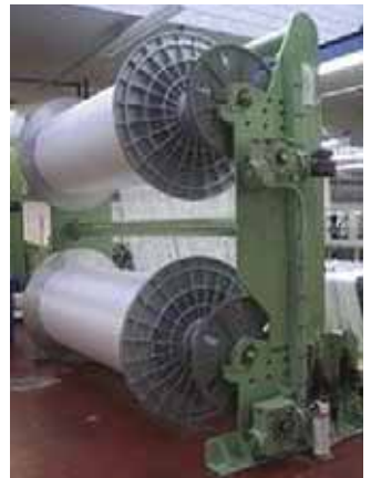
Weaving from Warp beam frame.
