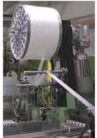
Controlled thread bobbin for the weaving of trade labels and written characters.
