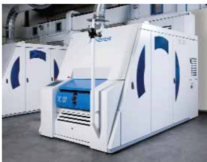
Truetzschler Card TC 7 with TCC card clothing accessories.
