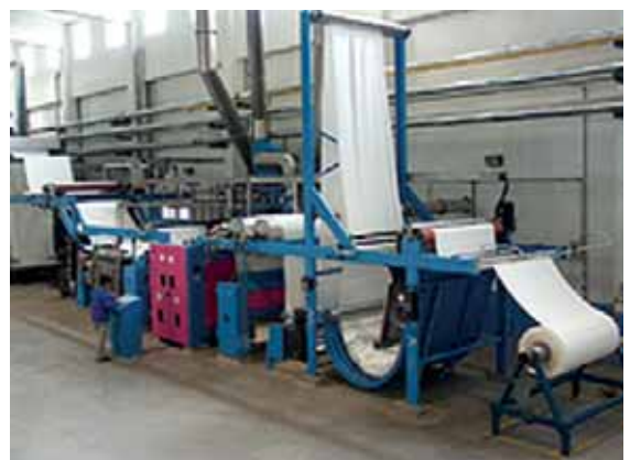
Finishing line with Osthoff Singeing Unit.
