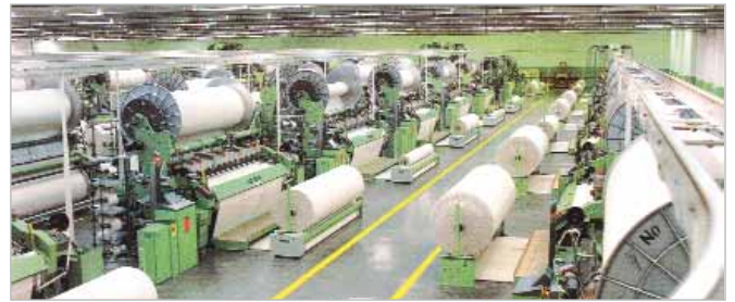
View in the weaving room of Indus Home Ltd. with the 48 Dornier air-jet terry weaving machines in production.
