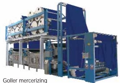
Goller mercerizing machine shown with denim application
