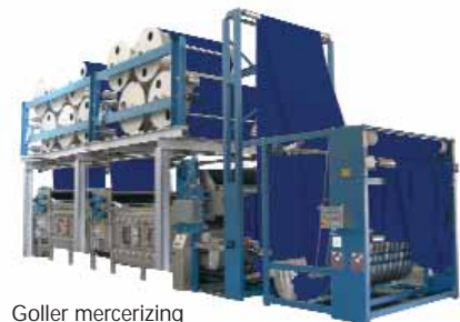
Goller mercerizing machine shown with denim application
