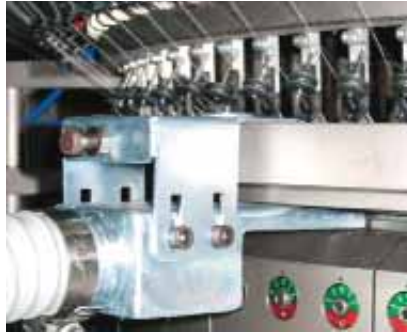
Suction nozzle placed on the dry zone of the needle to extract oil and lint.
