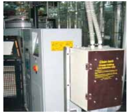
Extractors installed for a Mayer & Cie single jersey knitting machine.
