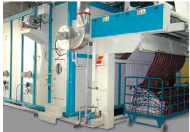
New Superwet (patented) steamer for reactive and pigment printing with temperature and humidity control system installed at Yunus Textile Mills Ltd.
