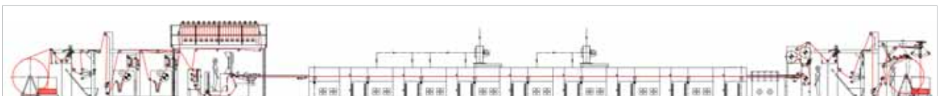
Figure 2: Brückner moist cross-linking line at Tianjin Tiange Textile Co. Ltd. in China.
