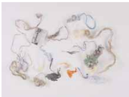
Fig. 3: Typical objects detected by 1-CCD colour sensors
