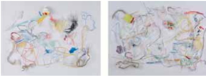
Fig. 6: Comparison of objects detected with a 3-CCD camera in a chute (left) and on a rotating cylinder (right).
