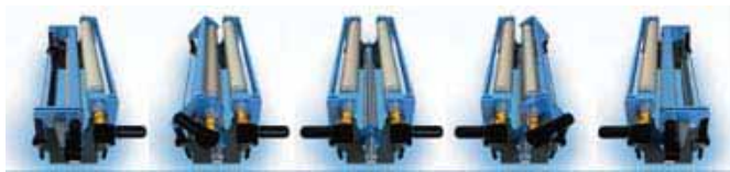
Fig. 5: Andritz Küsters neXcal twin, change of engraved roll .
