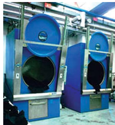
Essiccatoi: Rotating dryer tilting type for garments and "seamless" products.
