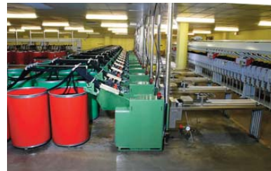
15 x S300 linked to a Schlafhorst 338E automatic winder with 60 spindles.
