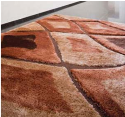
Super Shaggy-loop carpet with 2 x 50 mm cut pile and 2 x 20 mm loop pile woven face-to-face on the USP93.
