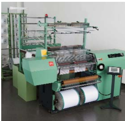
MDC - electronically controlled warp knitting machine for technical textiles.
