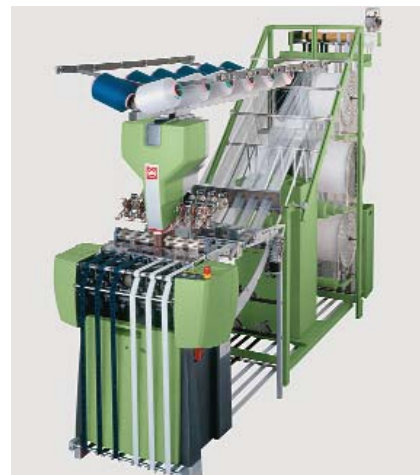
NH 53 - electronically controlled narrow fabrics loom.
