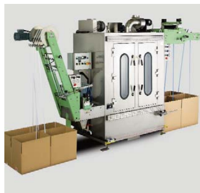
MFR 3A - narrow fabric pigment dyeing system.
