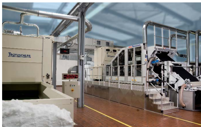
New Erko Carding System at the Fleissner Technology Center.
