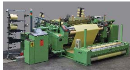
Dornier weaving machine, type PS, 220 cm wide, to manufacture ballistic fabrics)
