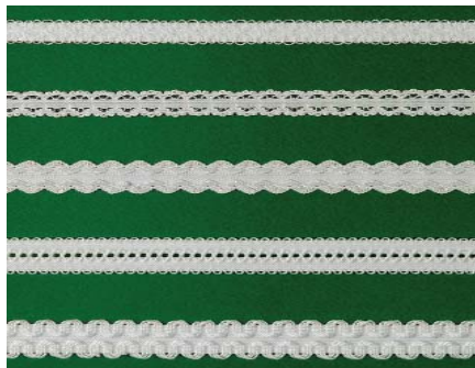
Elastic laces made on Comez crochet machines.
