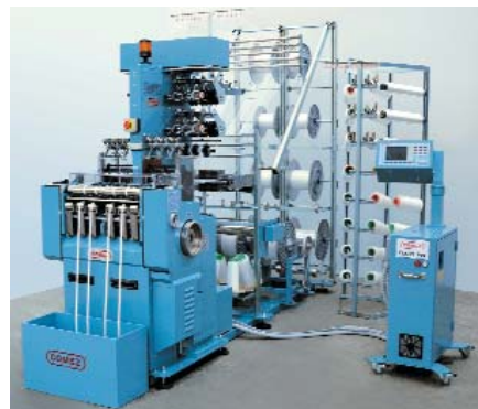
Electronic weaving needle loom Comez CLX-EL.
