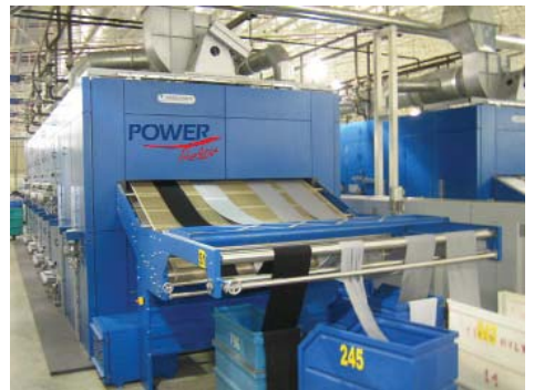
The more intense combination of suction and air circulation allows an absolutely homogeneous drying across the fabric width / fabric thickness and thus also an optimum fabric quality with the best achievable residual shrinkage.
