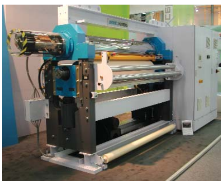
teXcal s-roll with a maximum line force of 400 N/mm.
